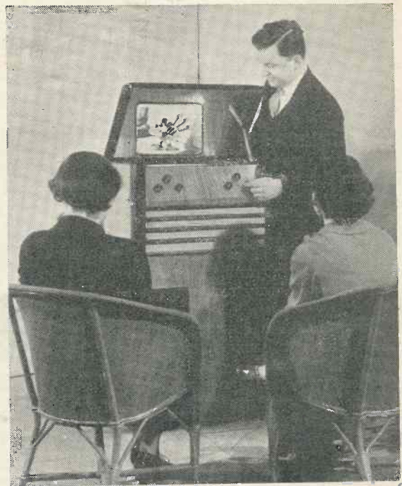
The Baird sound and vision receiver. Since this photograph was taken an additional control has been added.
